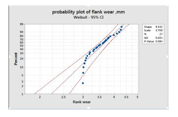
region of the straight lines and only a very few are out of the region when compared to the weibull probability plot. Hence flank wear in the present case follows normal distribution and the assumption has been proved.
