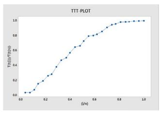
The reliability function for the tool life was derived using flank wear as the major phenomenon. The validation of the assumed flank wear distribution was done using statistical software MINITAB-16. The reliability of the cutting tool can be calculated with the derived reliability function with the help of the—Standardized normal probability tables.
